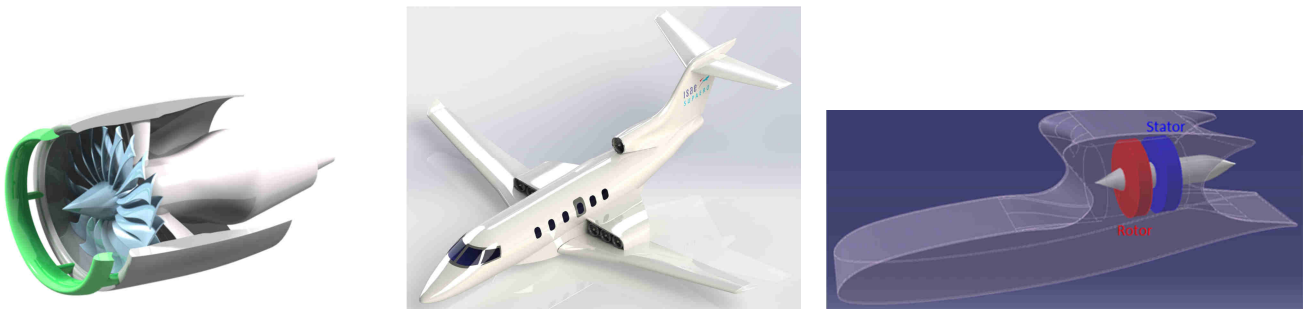
Fig.1. Slotted-inlet nacelle (left) and boundary-layer ingestion aircraft concept 3 (center and right)
